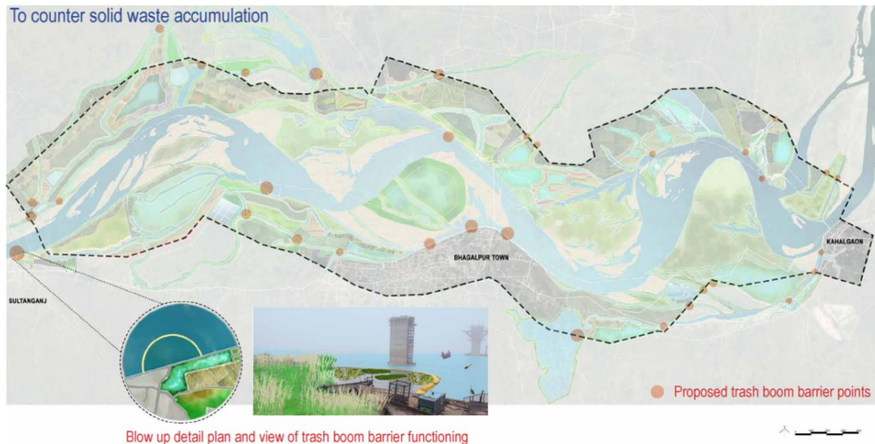
Figure 90 – Proposed locations for trash boom barriers across the sanctuary extent with a blow up detail highlighted for the location near Sultanganj ghat, Sultanganj. (Source - Author)
